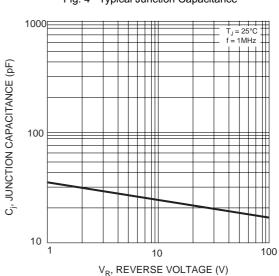
Fig. 4 Typical Junction Capacitance
